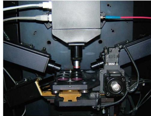
Figure 1. The confocal accessory
