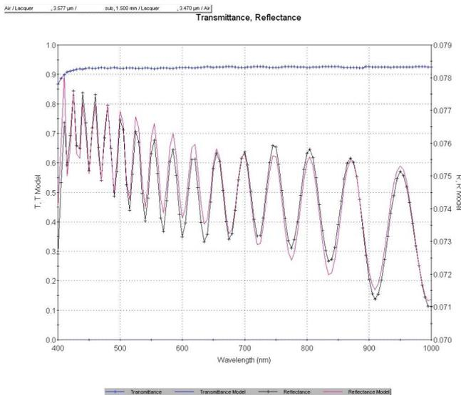
Figure 7. Ophthalmic lens, lacquer coated both sides. spectra shows T and R measurement at 10° measured at the edge of the lens. Overlaid on this in red is a model fitted for the lacquer.
